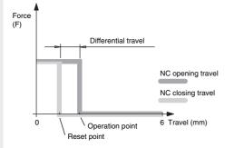
Contact blocks with snap action 5, 11. The pressure on the contact keeps constant while approaching to the snap point.
