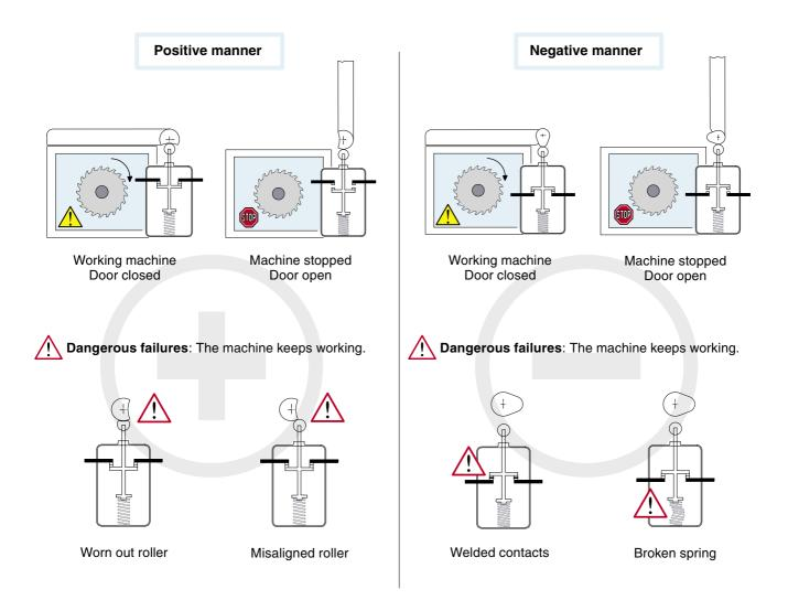
The positive manner avoid, with a preventive maintenance, the dangerous failures indicated above. On the contrary, the negative manner failures occurs inside the switch and are therefore difficult to be detected. With the positive manner, internal failures (welded contacts or broken springs) allows the opening of the contacts and therefore the machine stops.
