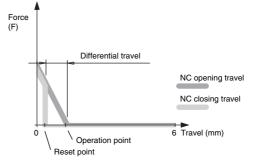
Contact blocks with snap action 2, 3. The pressure on the contact decreases while approaching to the snap point.
