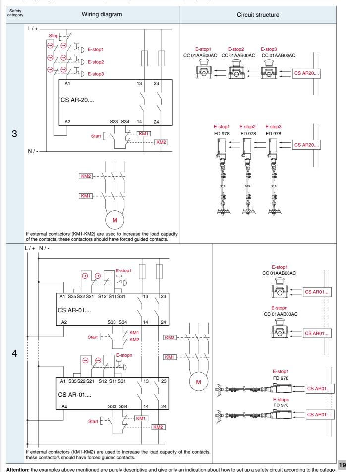
ries foreseen by standard EN 954-1. It is responsibility of the manufacturer to control that correct circuits are applied on each specific machine .
