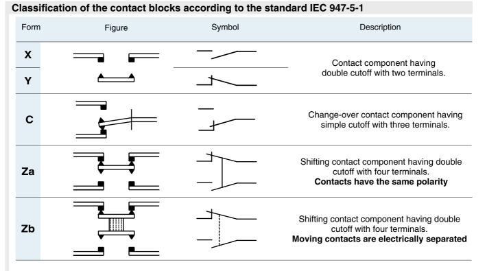
Symbol "+" between contact forms (e.g. X+X, Za+Za, X+X+Y, etc.) means that contacts have electrical separation between each other. The **electrically separated contacts allow** the application of different voltages and polarities between the contacts (fig. a).
