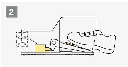
The foot must be completely inserted in order to lower the safety lever and push down the pedal actuator.
