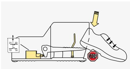
The safety lever prevents the pedal actuator from lowering when the foot is not completely inserted, thus preventing casual or accidental actuation.
